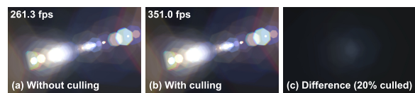
Figure 9: Culling low intensity flares can boost performance drastically (34% speedup here) with low visual impact.
