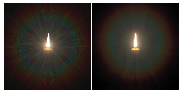
Figure 10: PSF applied using (left, 52.4 fps) billboards and (right, 30.2 fps) the convolution we propose. The results are substantially different for this candle. Using convolution, the horizontal needles of the ciliary corona blur out while the vertical needles remain unaffected.
